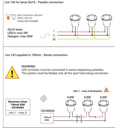
Lira 140 mains powered 198-264V 50/60Hz - Parallel connection
