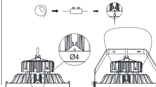
For any type of installation, it is recommended to secure the luminaire with a steel safety cable (not included)
